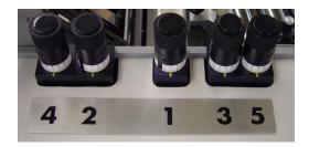
Exclusive, fast and accurate setup of folding roller pressure using the BaumQuick paperless gapsets
