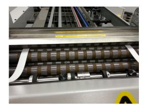
As you place each strip of paper into the proper fold rolls that you are calibrating the gapsets for, it is helpful to turn the gapset knob counter-clockwise until the strip of paper is being held lightly by the fold rolls.
