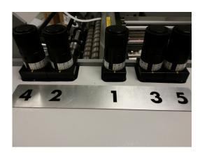
6. On all gapset knobs, using a 2mm allen wrench, tighten the set screws that hold the plastic binder plug so that the binder plug applies pressure to the gapset threaded rod. Tighten this set screw so that the plastic binder plug is actually "compressed" on the threads of the gapset rod threads. This step will ensure that the gapset knob does not turn as the rolls open and close as the sheets are passing through the fold roll bank.
