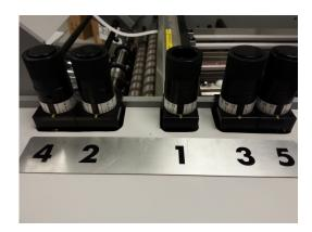
8. While holding the gapset knob so it does not turn, tighten the elastic stop nut located in the cavity of the gapset knobs slowly to ensure that it just contacts the gapset knob. This is done using a 1/2" or 13mm nut driver. Do this for all gapset knobs.
