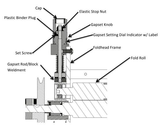
Adjusting fold rolls due to normal wear and tear on the folder is common. Recalibrating the fold rolls for this is very easy.
