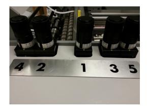
It is possible that you may have to turn the gapset knob to have the room to tighten this set screw on some of the gapset knobs. If you must turn the gapset knob to tighten this set screw, after you tighten this set screw as described, ensure that you turn the gapset knob back to a setting of 1.
