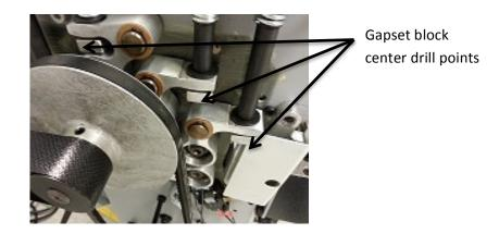
3. Due to tolerance stackup of components used in the gapset assemblies, there will be a variation as to where the max setting of each gapset knob will be. Some gapset knobs may not rotate a full 360 degrees and stop at a setting of 13. Some gapset knobs may rotate beyond 360 degrees and stop at a setting greater than the intended max setting of 15.
