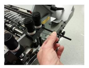
7. Each gapset indicator dial has a label with indication of settings from 1-15, with an open area in which the label does not wrap around the entire ring. Turn all of the gapset knob counterclockwise until the gapset indicates halfway in between the 1 & 15 indicators.
