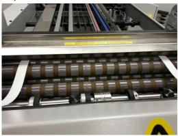
4. Calibrating the fold roll gap/pressure.
